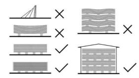
Valchromat panels must be stored in a covered area, protected from sunlight and rain, with a flat and horizontal base. The pallets must be placed on supports with sufficient height ( $\geq 8$  cm) to allow easy access with a forklift. The maximum distance between supports should not exceed 800 mm.
